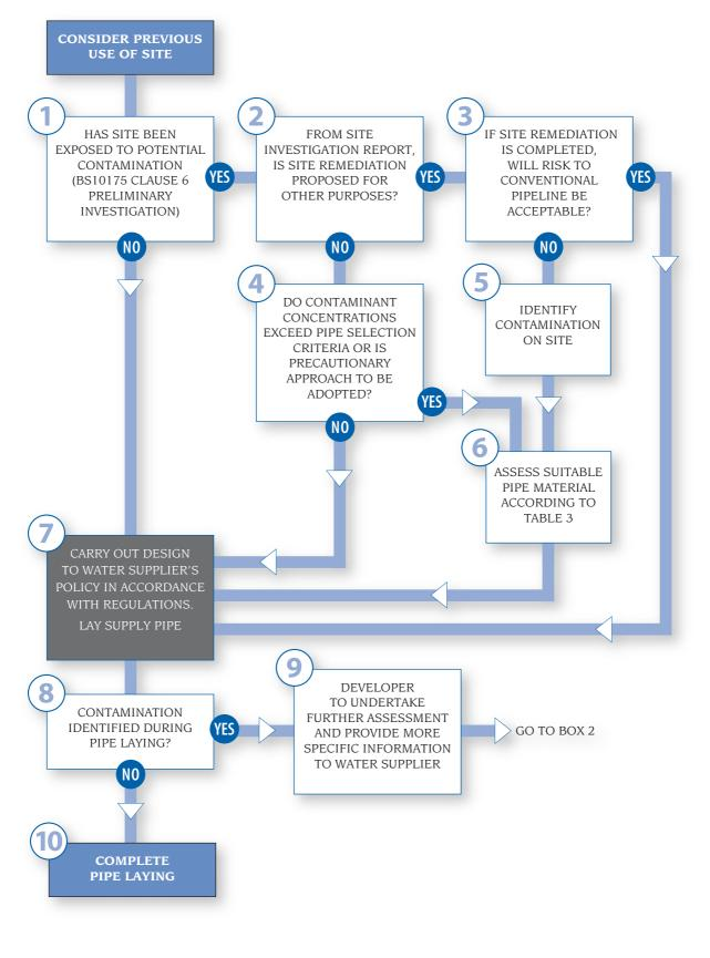
Figure 1: Investigation of contaminated land for pipe material selection and installation
